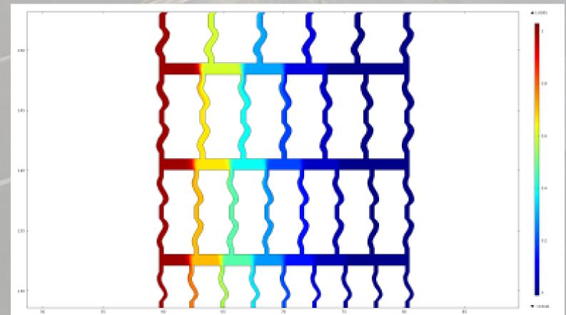
• Output channel may be too small and cause backup/turbulence in cell culture chambers
